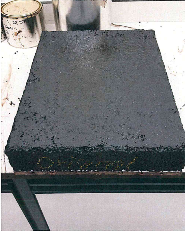
Figure 2-2: Slab after application of Original Formulation
